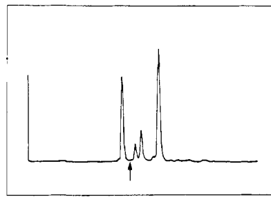
Figure 2. HPLC trace of the I_2 -catalyzed mixture of the retinol palmitates. The separation technique is described under Materials and Methods. The order of elution is the 13-cis, 9-cis, 13-cis, 9-cis, and all-trans isomers. An arrow points to where the 11-cis would appear.
